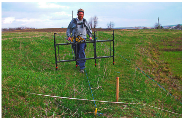
Fig. 5. 4-channel Förster magnetometer with a local grid system in use at Chișcăreni XIV (Photo by S. Țerna)
