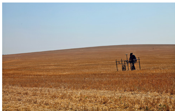
Fig. 6. 5-channel Sensys magnetometer with a GPS-system in use at Stolniceni I (Photo by S. Țerna)
