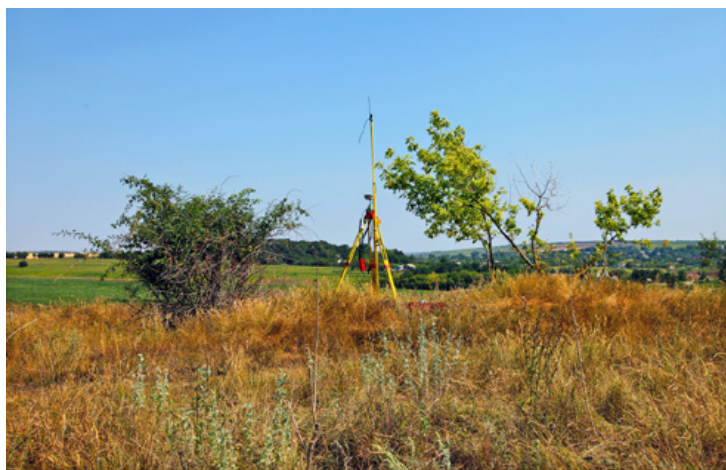
Fig. 5. 4-channel Förster magnetometer with a local grid system in use at Chișcăreni XIV (Photo by S. Țerna)
