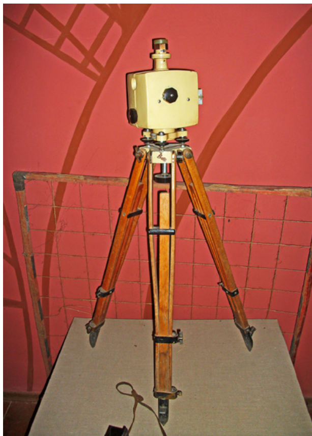
Fig. 4. M-27 magnetometer often used for prospection of the Tripolye sites. Here – on display in the Legedzine Museum of Trypillia culture, Ukraine (Photo by S. Ţerna)
